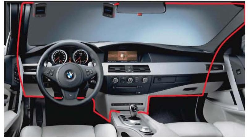
4. Organize the wire as shown above. Simply tuck into headliner and follow down which ever pillar takes you easiest to your power source. When coming down pillar simply remove the weather stripping and tuck behind and then put back in place.
