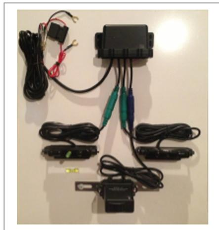
The Engine components include the CPU/Wing Box, 2 Laser diffusers, 1 Radar Detector, wire harness to hook up to cars battery terminals. As well as the brackets, screws and zip ties for mounting.
