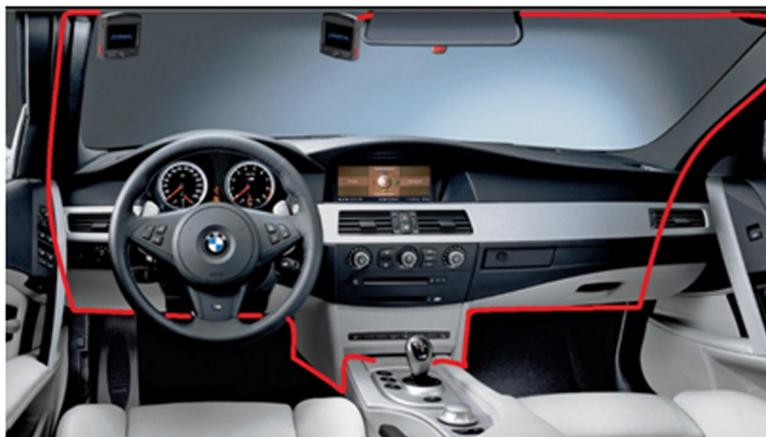
4. Organize the wire as shown above. Simply tuck into headliner and follow down whichever pillar takes you easiest to your power source. When coming down pillar simply remove the weather stripping and tuck behind and then put back in place.
